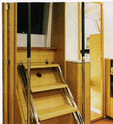
Full-height handholds are a useful feature either side of the companionway steps
