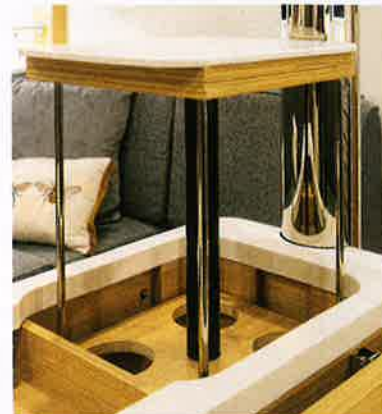
Hidden bottle-storage pops up from the forward end of the saloon table
