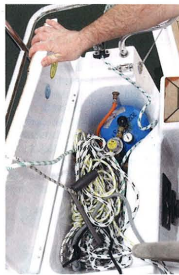
When asked about the risk of the gas bottle regulator being torn off by a line, Hanse replied that it now offers halyard bags to prevent it happening
